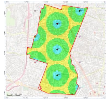
Fig. 2. Simulation result of SS-RSRP value in scenario 1
