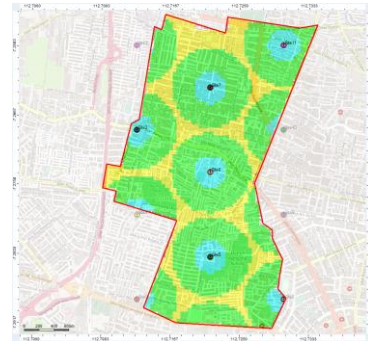
Fig. 10. Simulation result of SS-RSRP value in scenario 3
