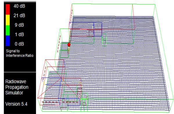
Fig. 17. Simulation results of 1 FAP SIR parameters 3D display
