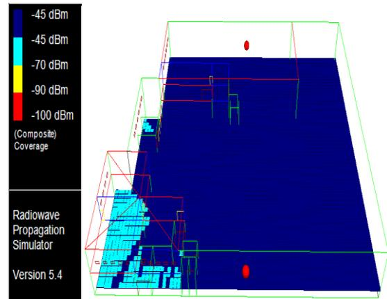
Fig. 8. Composite coverage result in second scenario in 3D view
