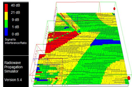
Fig. 14. Simulation results of the three SIR scenarios in 3D display
