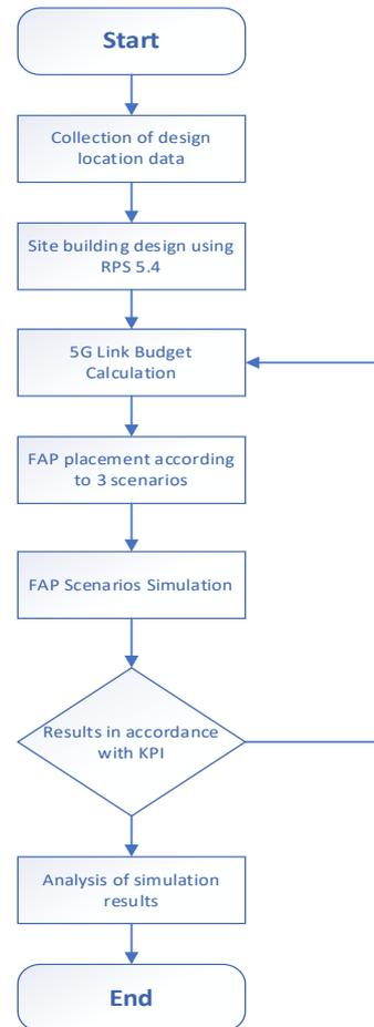
Fig. 1. Flowchart Design of 5G Indoor Coverage
