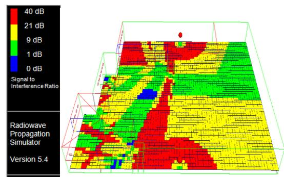
Fig. 10. SIR simulation result in second scenario in 3D view
